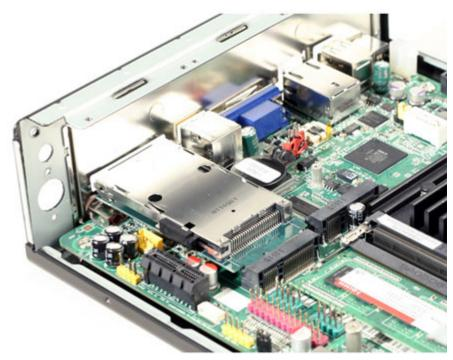
All Intel DN2800MT or Mitac PD10BI boards have a cutout slot for inserting 34mm Express Card.
